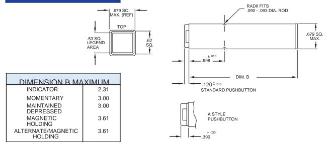
Tolerances: Unless otherwise specified - Fraction + 1/32", Note:Only standard and "A" style pushbuttons .XX+.01, XXX + .005
